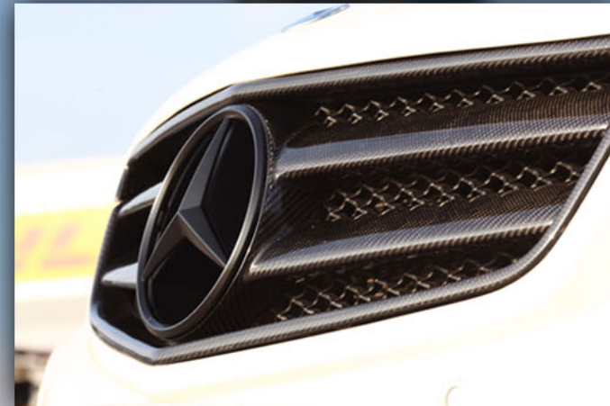
■ Carbon Front Grill P/N: Z 207 2 OEM A300
